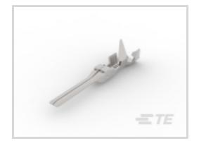
Power Contact Type: Contact Operating Voltage: 600 VDC Contact Mating Area Plating Material: Pre-Tin Wire Size: 20 – 18 AWG
