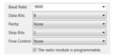
**Note** Failure to enter AT Command Mode is typically due to baud rate mismatch. Ensure that the **Baud** setting on the **Add radio device** window matches the interface data rate of the RF module. By default, the BD parameter = 9600 b/s.
