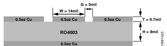
Figure 23. Probe Matrix Board (Cross Sectional View)
