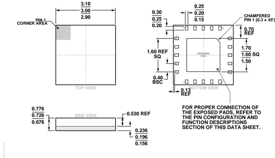
Figure 24. 20-Terminal Land Grid Array [LGA]
