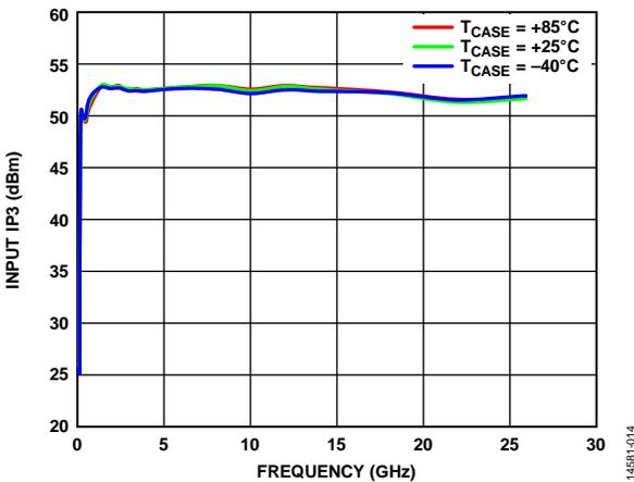
Figure 14. Input IP3 vs. Frequency over Temperature
