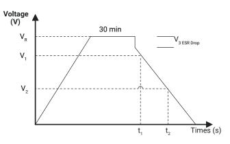
I - Discharge Current [mA], 4 \* C \* VR VR - Rated Voltage
