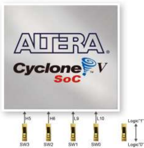
Figure 3-8-16 Connections between the slide switches and the Cyclone V SoC FPGA
