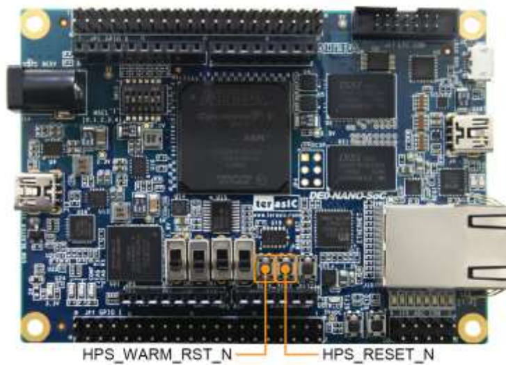
Figure 3-3-11 HPS cold reset and warm reset buttons on Atlas-SoC
