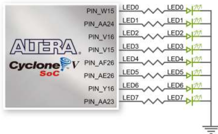
Figure 3-9 Connections between the LEDs and the Cyclone V SoC FPGA
