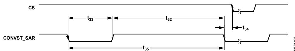
Figure 5. SAR ADC Timing Diagram
