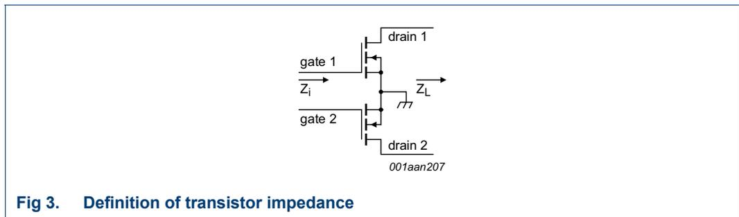
Fig 3. Definition of transistor impedance
