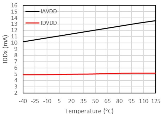
Figure 7-21. Supply Current vs. Temperature
