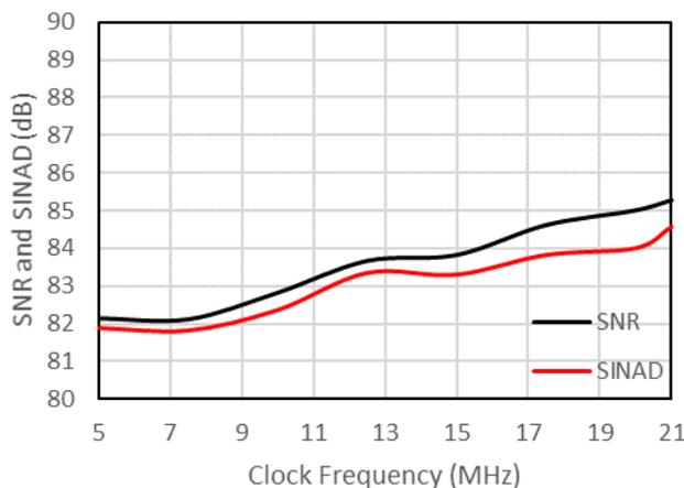
Figure 7-11. SNR & SINAD vs. Clock Frequency
