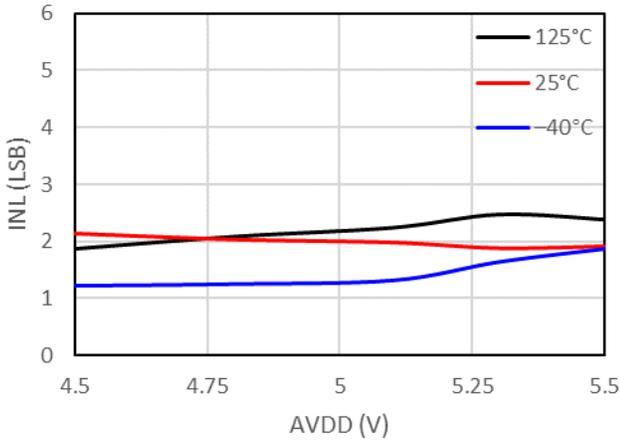
Figure 7-25. INL vs. High-side Supply Voltage
