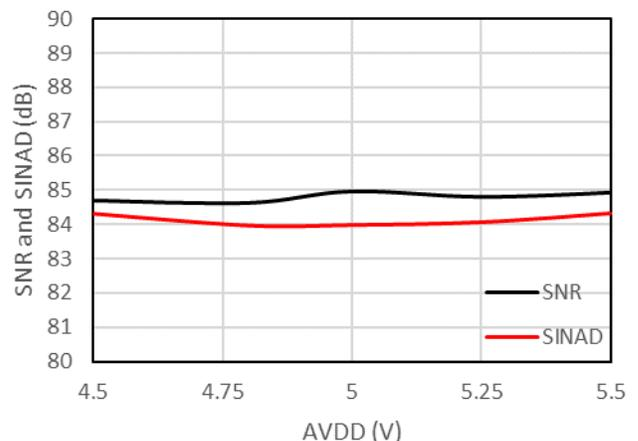
Figure 7-10. SNR & SINAD vs. High-side Supply Voltage
