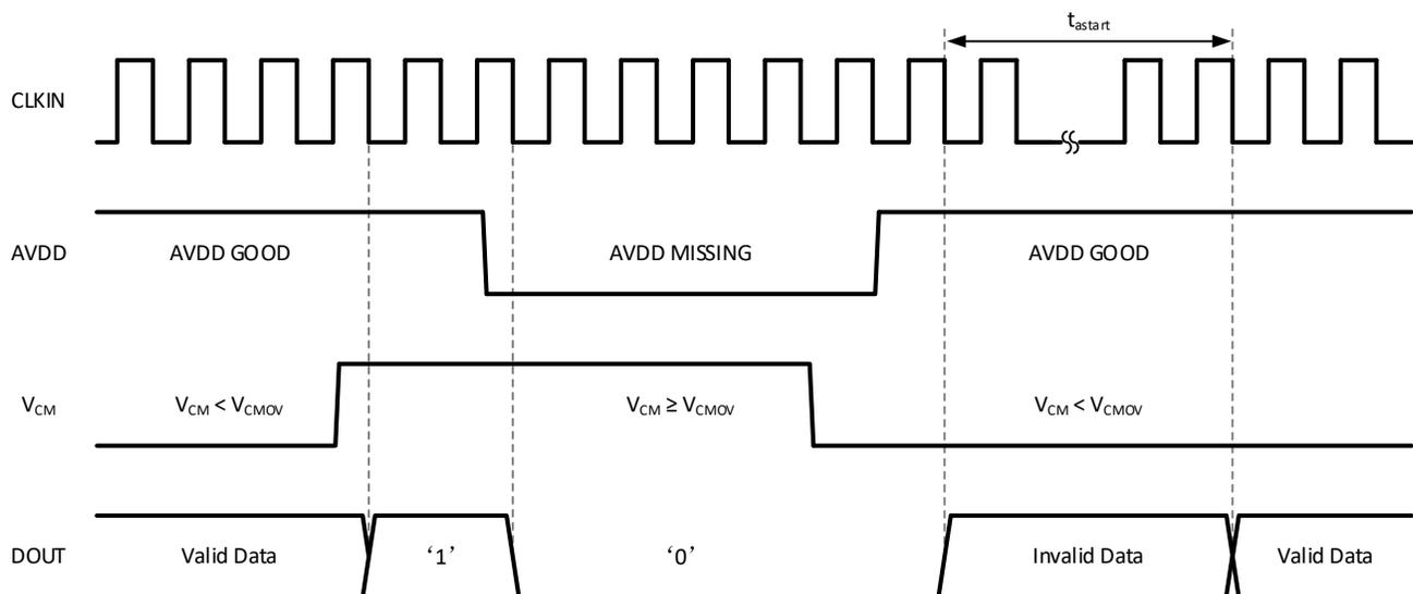
Figure 8-5. CA-IS1305x Over-range Output Waveforms
