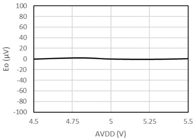
Figure 7-5. Offset Error vs. High-side Supply Voltage
