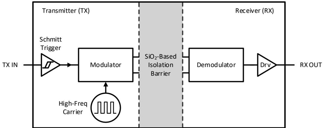
Figure 8-2. Block Diagram of the Isolation Channel
