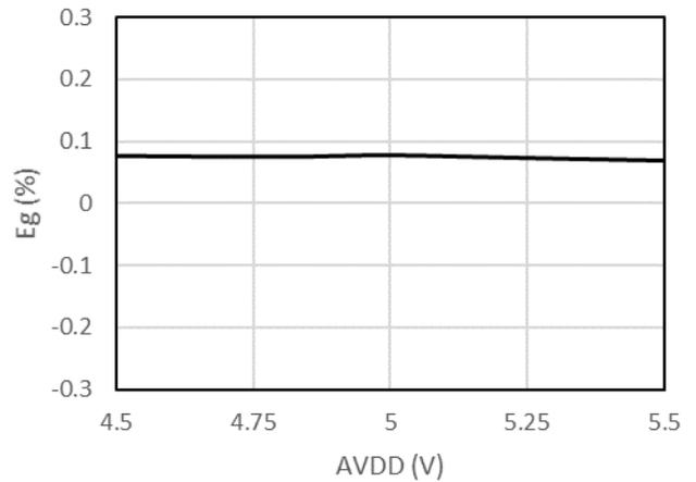
Figure 7-2. Gain Error vs. High-side Supply Voltage
