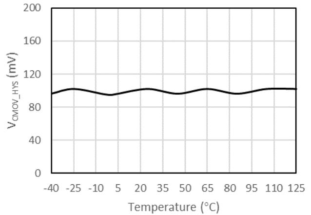
Figure 7-8. Hysteresis of common-mode over-voltage threshold vs. Temperature
