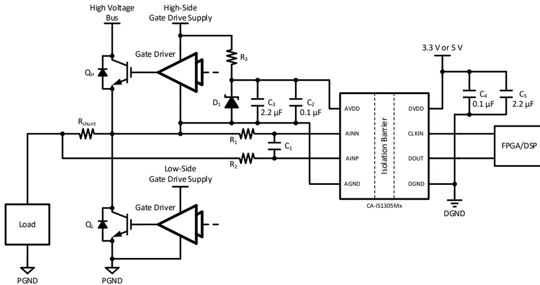
Figure 9-1. Typical Application for 1-phase Current Sensing
