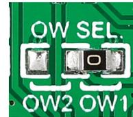
The board features an 0W jumper [zero ohm resistor] that allows you to choose between two available pins for the 1-Wire interface.
