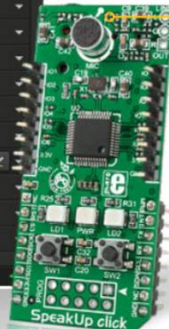
When you put it to work, it listens to what you're saying, matches the sound to one of the pre-recorded commands, and triggers the specified action which the on-board MCU executes.
