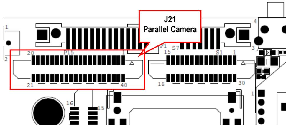
Figure 18 – COM Carrier Board, Parallel Camera Interface Connector
