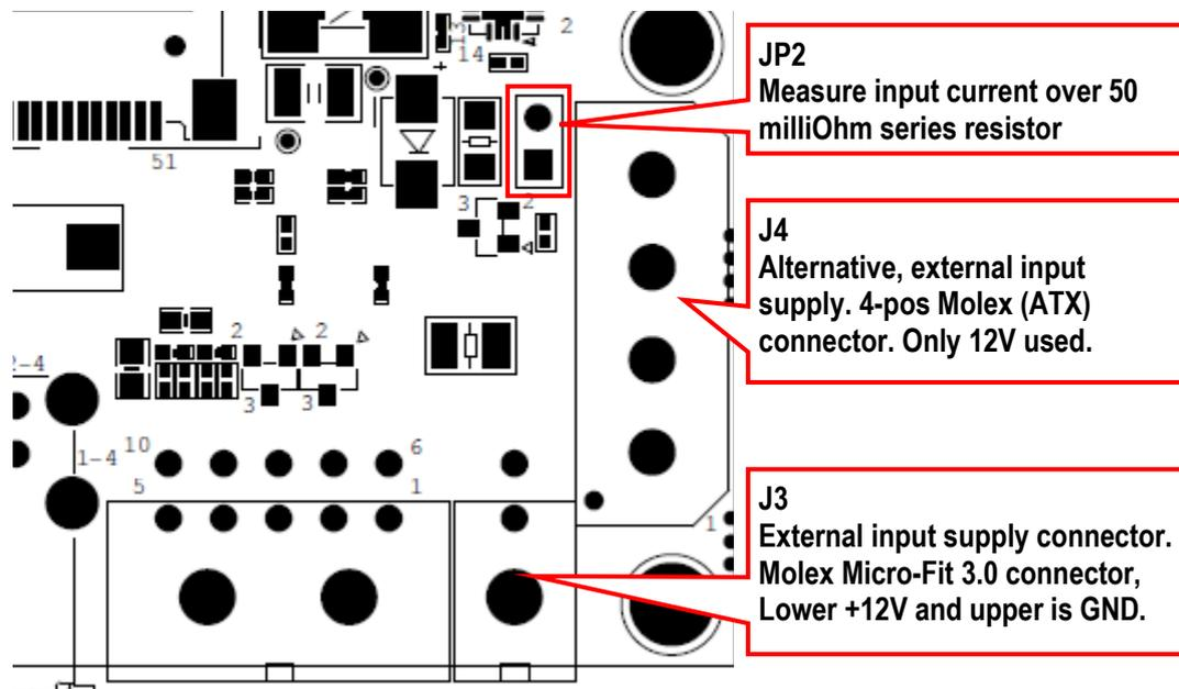
Figure 4 – COM Carrier Board, Power Supply Connectors
