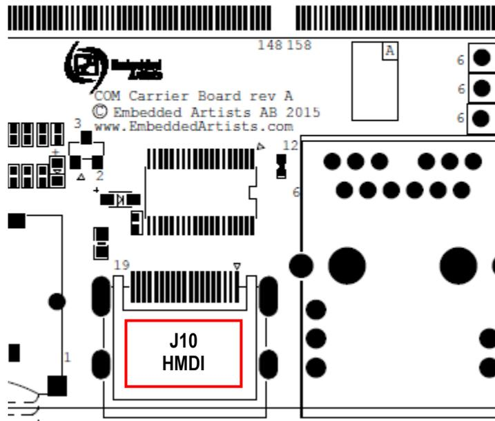
Figure 10 – COM Carrier Board, HDMI Connector
