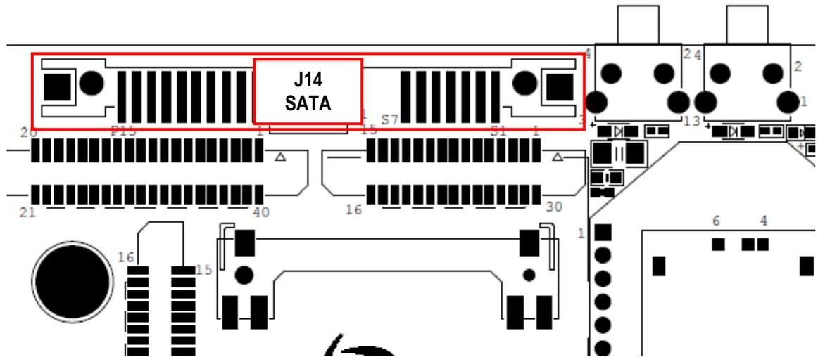
Figure 13 – COM Carrier Board, SATA Interface Connector
