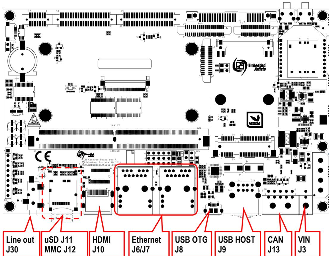
Figure 2 – COM Carrier Board, Main External Interface Connectors
