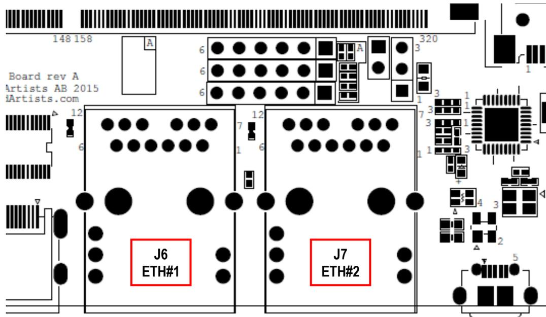
Figure 8 – COM Carrier Board, Dual Ethernet Connectors
