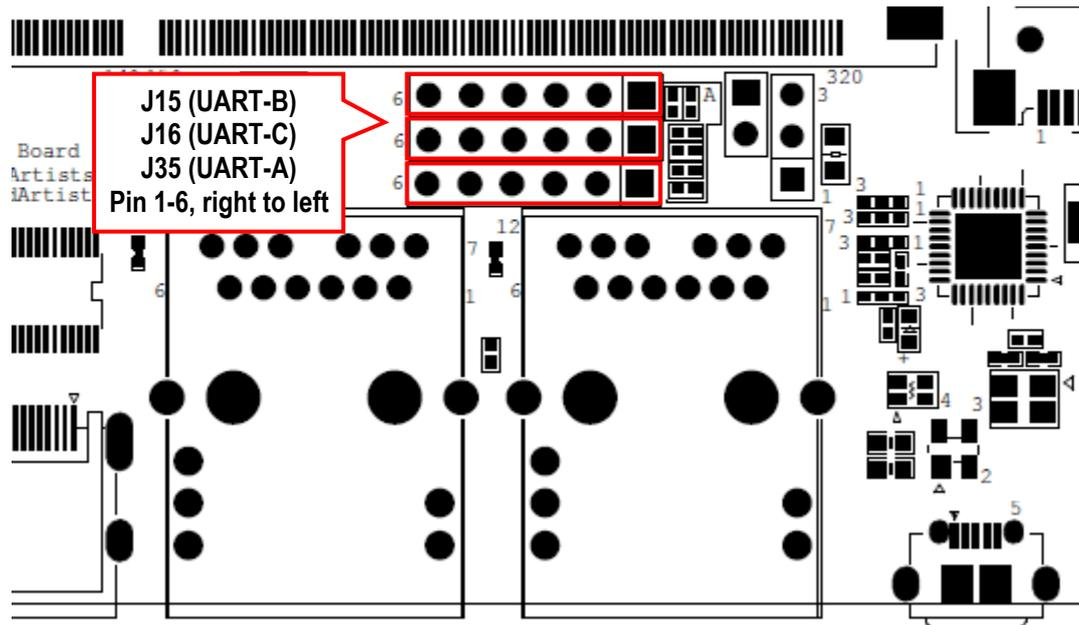
Figure 14 – COM Carrier Board, UART Interface Connectors
