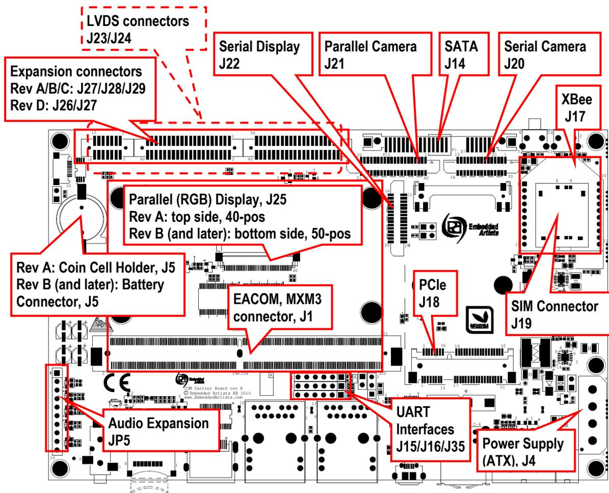
Figure 3 – COM Carrier Board, Main Internal Connectors
