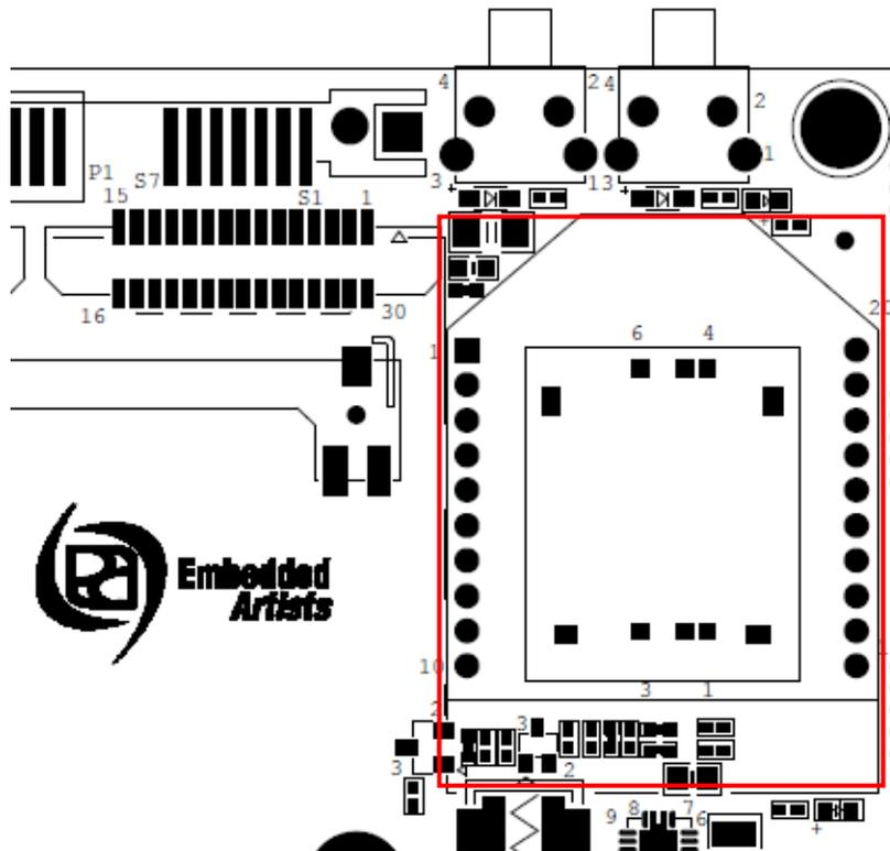
Figure 15 – COM Carrier Board, XBee Interface Connector
