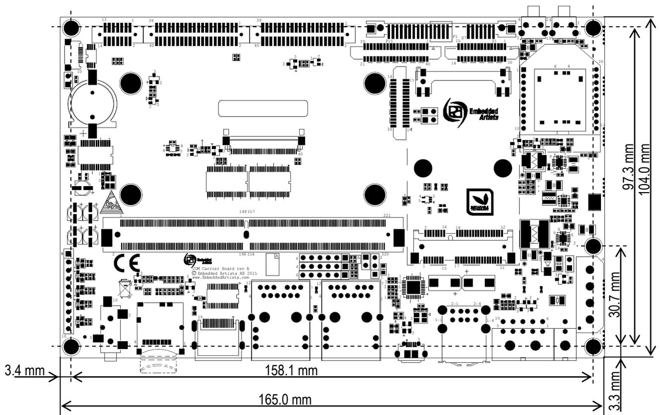
Figure 27 –COM Carrier Board Mechanical Outline
