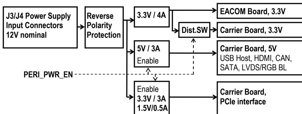
Figure 5 – COM Carrier Board, Power Supply Chain
