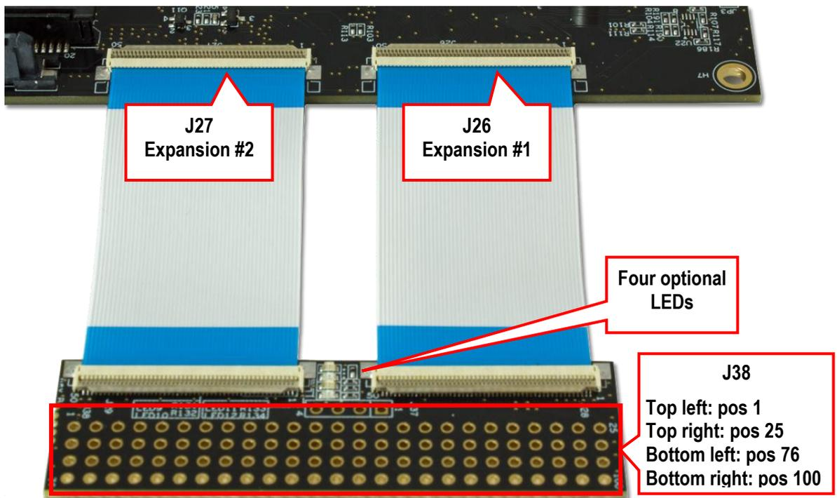
Figure 25 – COM Carrier Board, Expansion Breakout Board
