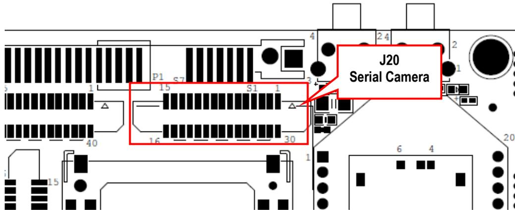
Figure 17 – COM Carrier Board, Serial Camera Interface Connector
