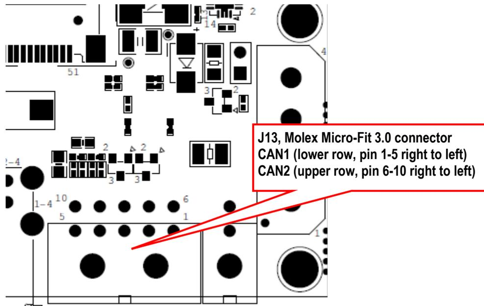
Figure 12 – COM Carrier Board, CAN Interface Connector
