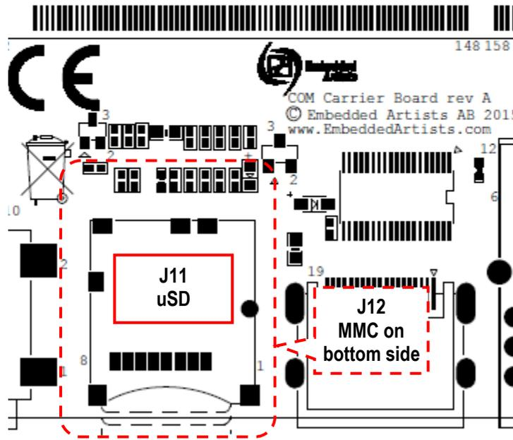
Figure 11 – COM Carrier Board, uSD/MMC Connectors
