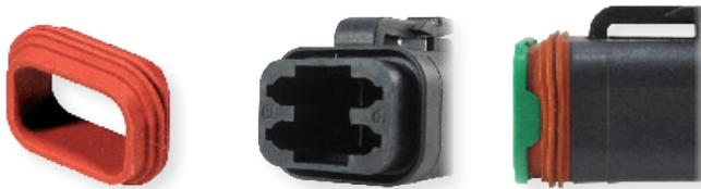
The DT P012 plugs provide enhanced front seal retention resulting in an ultra tight environmental seal. The enhanced seal retention keeps the seal in place during mating and unmating. The P012 modification requires an enhanced P012 wedge lock. The DEUTSCH P012 modification is available in 2, 3, 4, 6, 8, and 12 cavity arrangements. P012 plugs have a black connector body except for the 8 and 12 cavity arrangements, where the color is based on the key.
