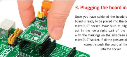
Once you have soldered the headers your board is ready to be placed into the desired mikroBUS™ socket. Make sure to align the cut in the lower-right part of the board with the markings on the silkscreen at the mikroBUS<sup>™</sup> socket. If all the pins are aligned correctly, push the board all the way
