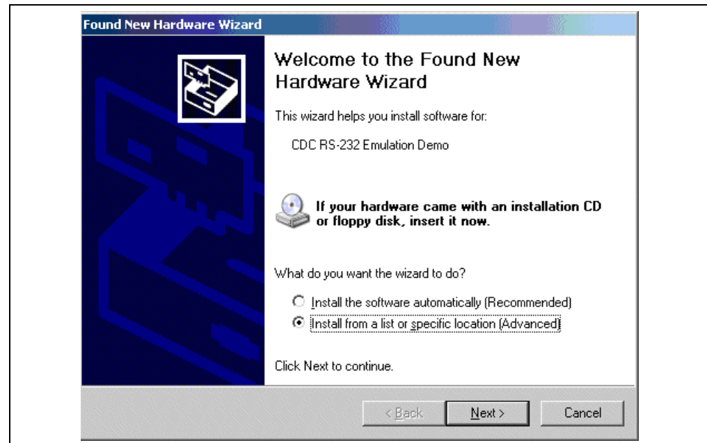
FIGURE 2-14: INSTALLING USB *.inf FILE ON PC – SCREEN 1
