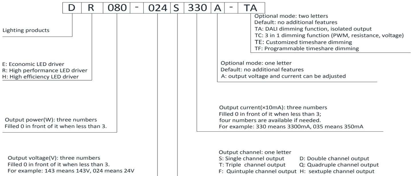
For example: DR080-024S330A-TA means: high performance LED driver; output power 80W; output voltage 24Vdc; output current 3300mA; single output; output voltage and current can be adjusted; with DALI dimming function and isolated output.
