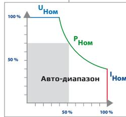
Both power classes reduce the output power automatically when the input supply is low, so the 1.5 kW models can still provide 1 kW power with an input supply of 100...150 V<sub>AC</sub> and the 3 kW models can still provide 2.5 kW at 180...207 V<sub>AC</sub>.
