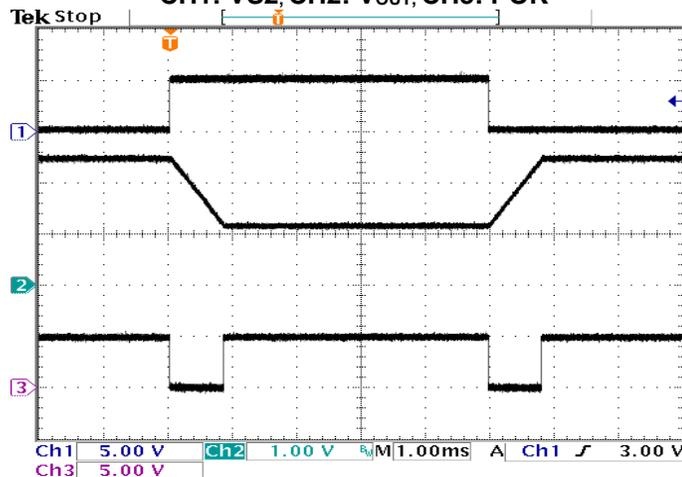
**$V_{OUT}$  Scaling with VID Codes at  $V_{IN} = 3.3\text{ V}$**
