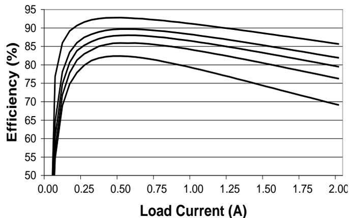
Top to Bottom:  $V_{OUT} = 2.5\text{ V}, 1.8\text{ V}, 1.5\text{ V}, 1.2\text{ V}, 0.8\text{ V}$
