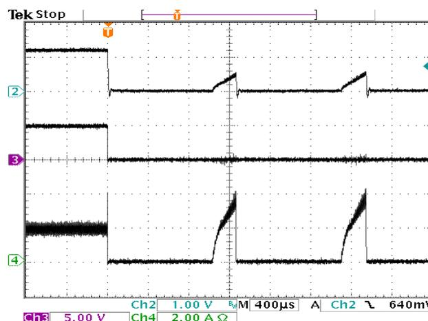
Output Over Load at No Load ( $V_{IN} = 5\text{ V}$ ,  $V_{OUT} = 1.2\text{ V}$ )
