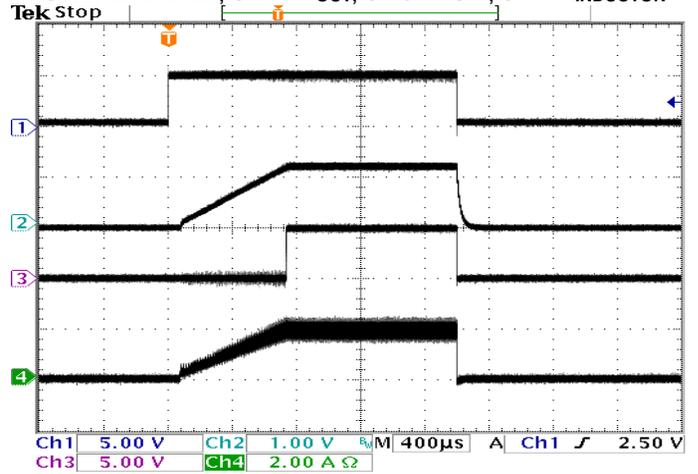
Output Over Load at No Load ( $V_{IN} = 5\text{ V}$ ,  $V_{OUT} = 1.2\text{ V}$ )
