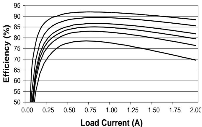
Top to Bottom:  $V_{OUT} = 3.3\text{ V}, 2.5\text{ V}, 1.8\text{ V}, 1.5\text{ V}, 1.2\text{ V}, 0.8\text{ V}$
