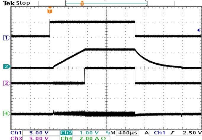
**Power Up/Down at  $0.6\ \Omega$  Load ( $V_{IN} = 5\text{ V}$ ,  $V_{OUT} = 1.2\text{ V}$ )**
