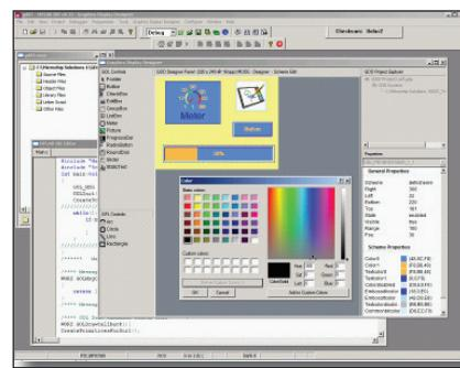
The Microchip Graphics Display Designer (GDD) is a visual design tool that provides customers with a quick and easy way of creating Graphical User Interface (GUI) screens for graphical interface applications on Microchip MCUs.
