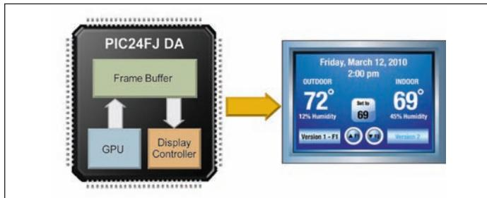
The PIC24F DA family makes it easy and cost-effective to add advanced graphics to your application by eliminating the need for external frame buffers or display controllers.
