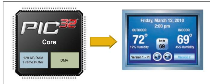
Microchip's PIC32 line of 32-bit microcontrollers offers 80 MIPS and high performance DMA to render graphics directly to displays. This enables PIC32 devices to drive a display without an external graphics controller.
