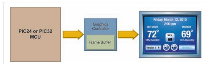
**The Solomon Systech SSD1926 Graphics Controller** has hardware graphics acceleration to free up the MIPS of the PIC MCU. This controller includes a SD Card interface and JPEG decode engine as well as 256 KB RAM. The Graphics PICtail™ Plus SSD1926 Board (AC164127-5) includes serial Flash for data storage and interfaces to either Explorer 16 or PIC32 Starter Kits.
