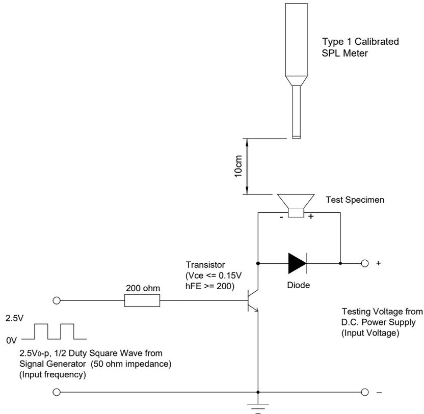
Figure 1. Test Setup
