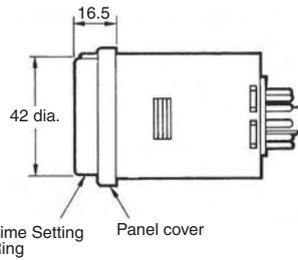
Dimensions with Front Connecting Socket
