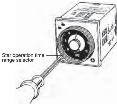
The time required for switching (0.05, 0.1, 0.25, or 0.5 second) from the star operation to the delta operation of the H3CR-G can be selected with the star-delta transfer time selector at the lower right corner of the front panel.
