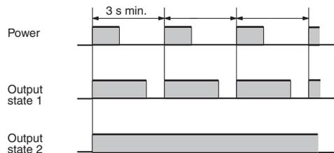
After the forced reset function of the H3CR-H is activated, an interval of 3 s minimum is required to activate the forced reset function again. If the forced reset function is activated repeatedly with an interval of shorter than 3 s, the internal parts of the H3CR-H may deteriorate and the H3CR-H may malfunction.
