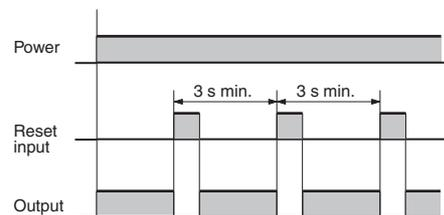
If it is required that the output be turned on repeatedly with an interval of shorter than 3 s, consider use of the H3CR-A in mode D (signal OFF-delay).
