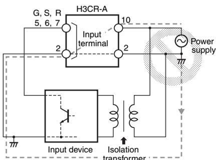
The H3CR-A□/-A□S/AP's power supply terminal 2 is a common terminal for input signals to the Timer. Do not disconnect the wires on terminal 2, otherwise the internal circuitry of the Timer will be damaged.
