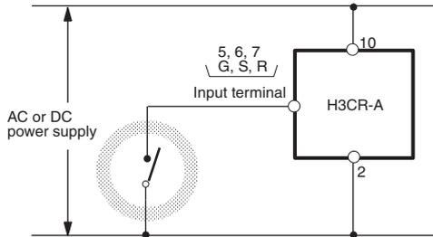
Do not connect a relay or any other load between input terminals, otherwise the internal circuit of the Timer will be damaged due to the high-tension voltage applied to the input terminals.
