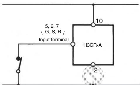
Make sure that the voltage is applied within the specified range, otherwise the internal elements of the Timer may be damaged.
