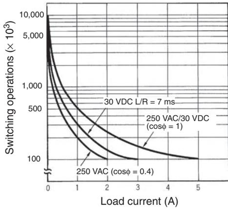
Reference: A maximum current of 0.15 A can be switched at 125 VDC (cosφ = 1) and a maximum current of 0.1 A can be switched if L/R is 7 ms. In both cases, a life of 100,000 operations can be expected. The minimum applicable load is 10 mA at 5 VDC for H3CR-H8L/H8RL and 100 mA at 5 VDC for H3CR-H8RL (failure level: P).
