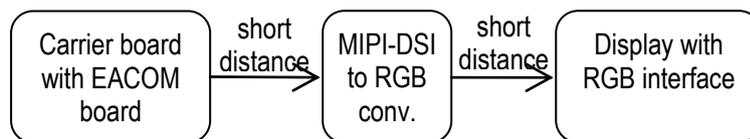
A good start for a MIPI-DSI to parallel RGB converter is Toshiba's TC358762XBG.
