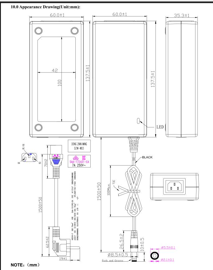
1) WIRE TYPE: VW-1 2468 80  $^{\circ}$ C 300V L=1500mm 2C 18AWG BLACK
