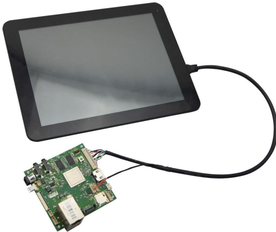
Figure 3 Connections between SABRE Lite and LCD8000-97C
