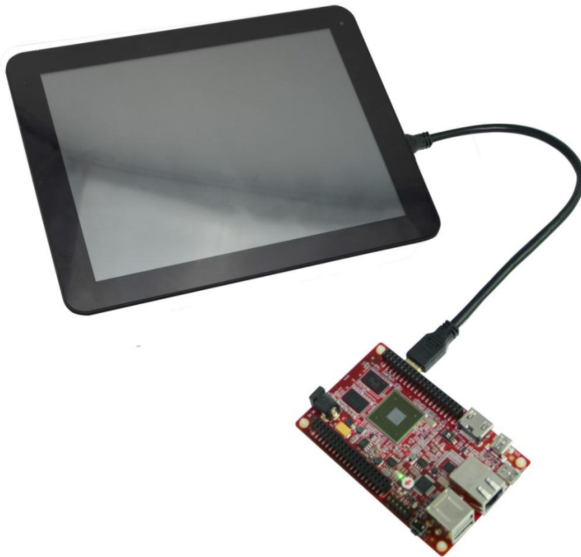
Figure 1 Connection between MarS Board and LCD8000-97C
