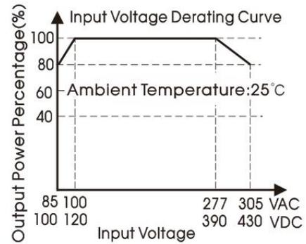
Note: 1. With an AC input between 85-100V/277-305VAC and a DC input between 100-120VDC/390-430VDC, the output power must be derated as per temperature derating curves;
