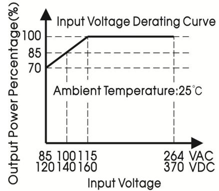
Note: With an AC input voltage between 85 -115VAC and a DC input between 120-160VDC the output power must be derated as per the temperature derating curves.
