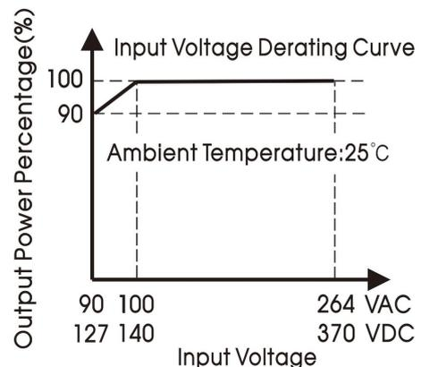
Note: With an AC input voltage between 90 - 100VAC and a DC input between 127 - 140VDC the output power must be derated as per the temperature derating curves.
