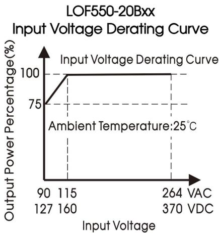
Note: With an AC input voltage between 90 - 115VAC and a DC input between 127 - 160VDC the output power must be derated as per the temperature derating curves
