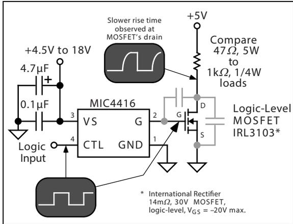
**FIGURE 5-5:** MOSFET Capacitance Effect at High Switching Frequency.
