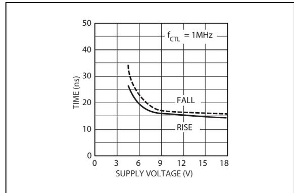
**FIGURE 2-11:** Rise and Fall Time vs. Supply Voltage.
