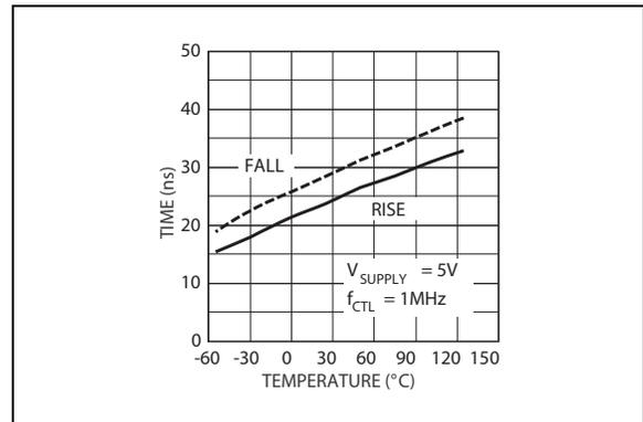
**FIGURE 2-12:** Rise and Fall Time vs. Temperature.
