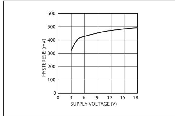
**FIGURE 2-16:** Control Input Hysteresis vs. Supply Voltage.
