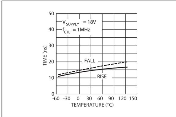
**FIGURE 2-13:** Rise and Fall Time vs. Temperature.
