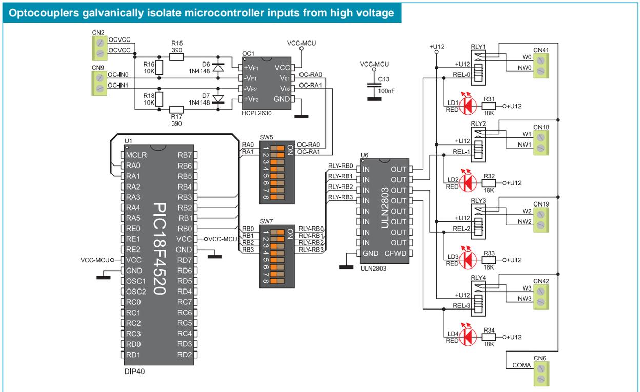
Figure 12-3: Relays and optocouplers and microcontroller connection schematic
