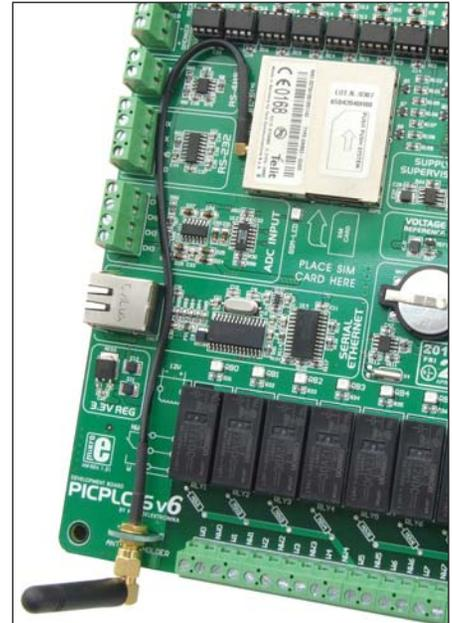
Figure 9-4: GSM module with antenna
