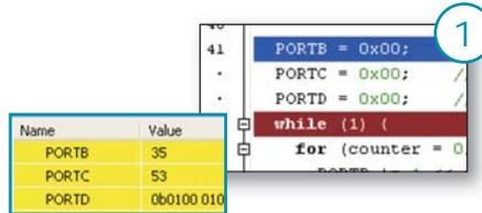
During operation, the program line to be executed next is highlighted in blue, while the breakpoints are highlighted in red. The *Run* command executes the program in real time until it encounters a breakpoint.
