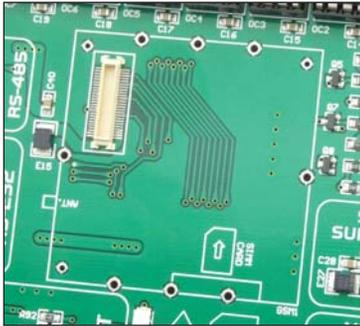
Figure 9-1: GSM connector
