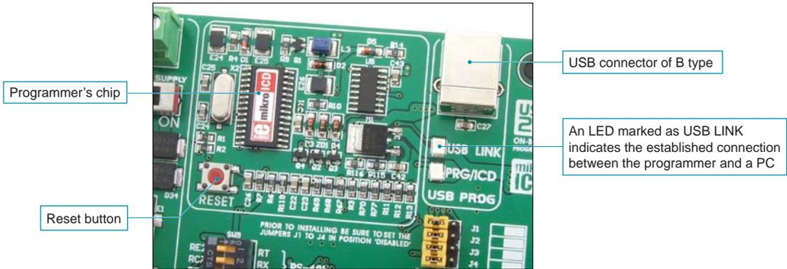
Figure 3-1: *PICflash* programmer
