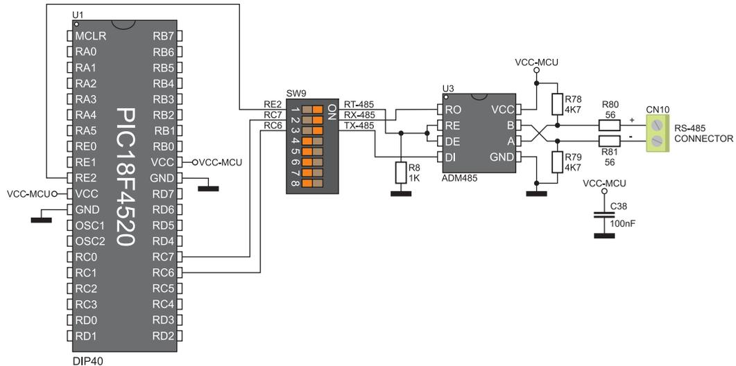
Figure 7-2: RS-485 module connection schematic
