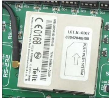
Figure 9-2: GSM module
