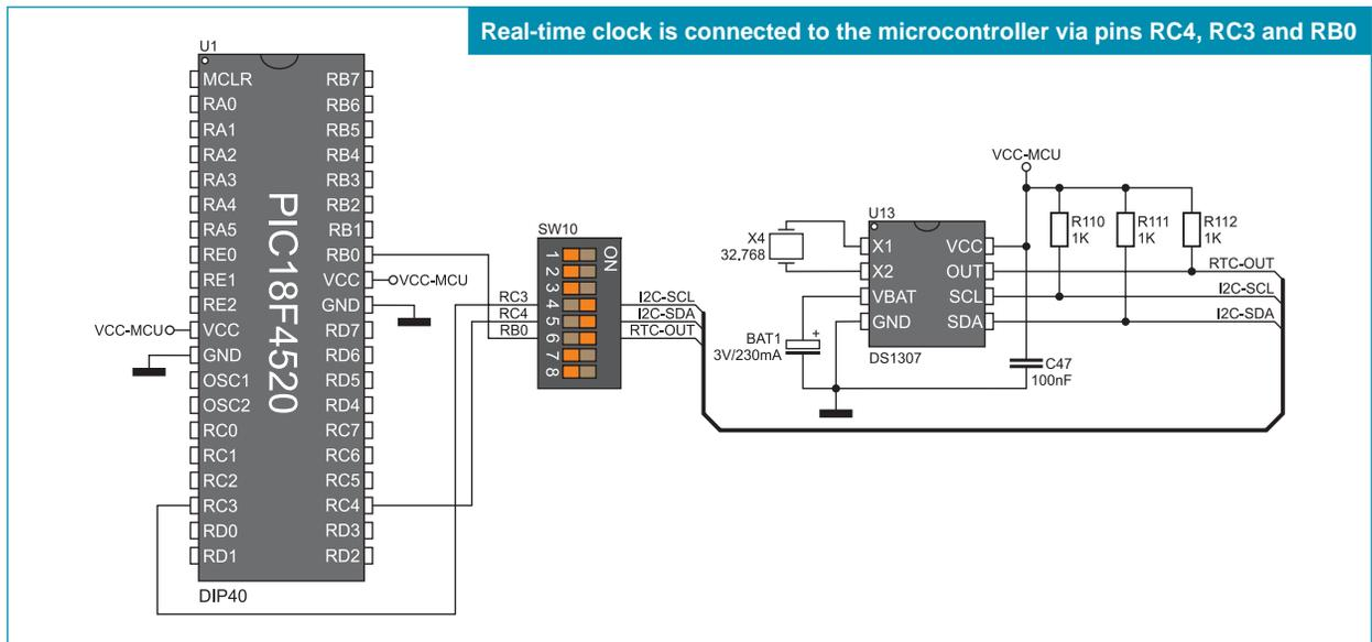
Figure 11-2: Real-time clock and microcontroller connection schematic
