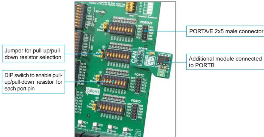
Figure 13-1: I/O ports
