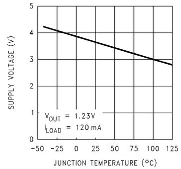
**$\overline{ON}$  /OFF Threshold Voltage**
