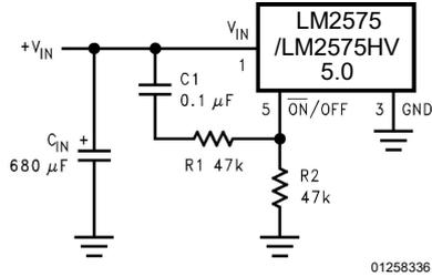
FIGURE 21. Delayed Startup
