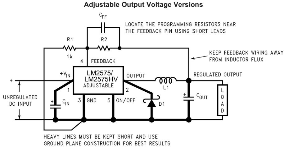
$$V_{OUT} = V_{REF} \left( 1 + \frac{R_2}{R_1} \right)$$
