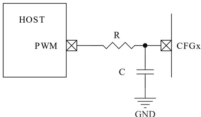
Note: Refer to Application Note 'Using PWM to Generate Analog Output (AN538)' for details about how to choose appropriate R and C values
