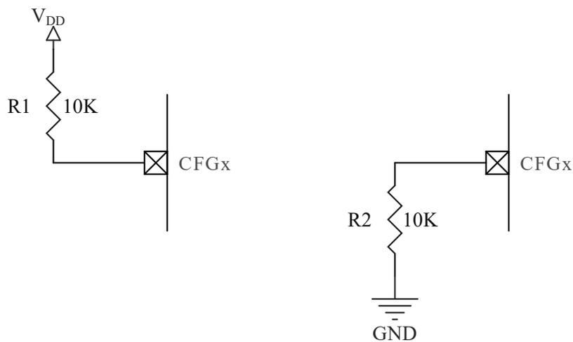
The pull-up/pull-down resistor is a precautionary recommendation, as MTCH1010 will not pull the  $CFGx$  neither to the  $V_{DD}$  nor to the  $GND$  during the operation.
