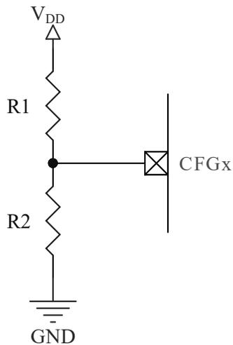
Note: Both  $R1$  and  $R2$  are recommended to be greater than 100K for lower power consumption
