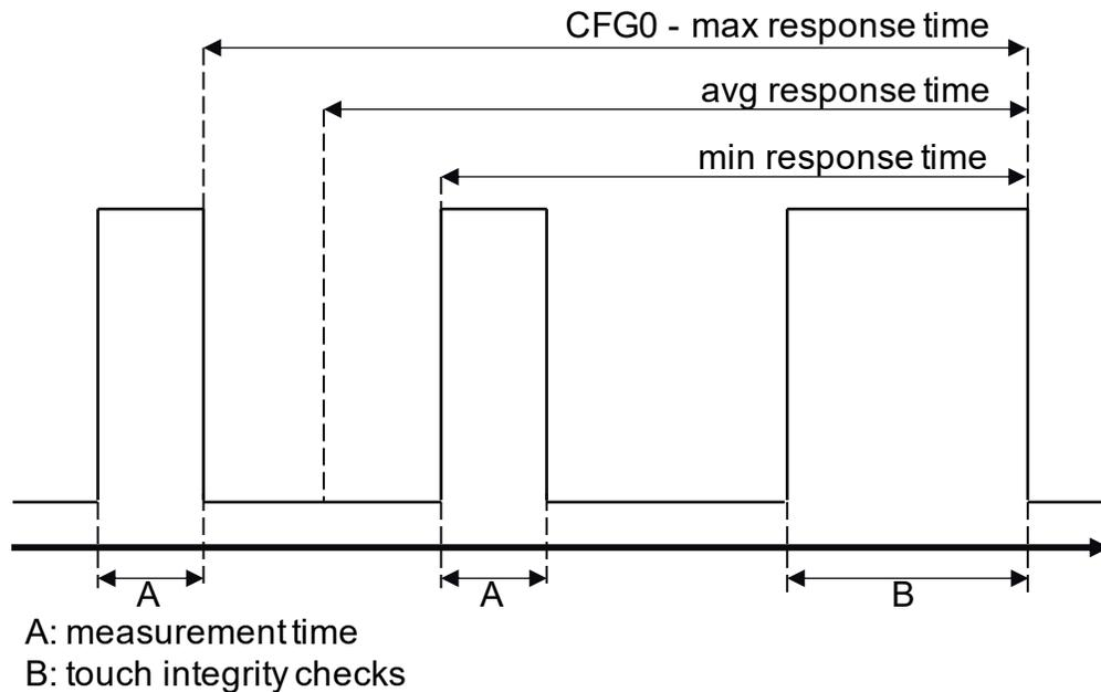
**Note:** During high noise, the response times may exceed the configured target, due to the automatic adjustment of oversampling period by frequency hopping. In the worst-case frequency selection, the maximum response time may be extended by 30%.
