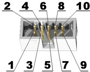
UEXT is connector for external plug-in modules.
