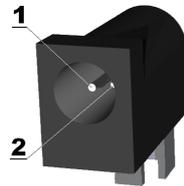
The PWR-CON connector is used to power the PIC-32MX board. You can use either AC or DC power supply. The range of each of the powering options are as follows (4.5 – 9)V for AC and (6 – 12)V for DC. Do not provide more voltage than these maximums values!
