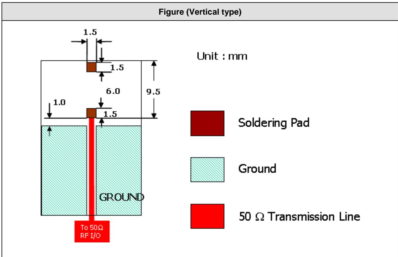
Antenna on Test Board ( FR4 Thickness 0.8mm)
