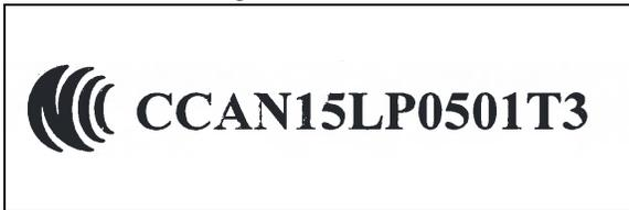
Due to the limited size of the RN4871, the NCC ID is not displayed on the module. Therefore, the outside of the device must also display a label referring to the enclosed module. This exterior label can use wording such as the following:
