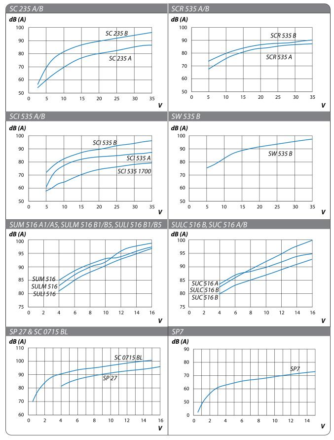
All measurements are made @ 12Vdc @ 1 meter in free air @ 21°C.
