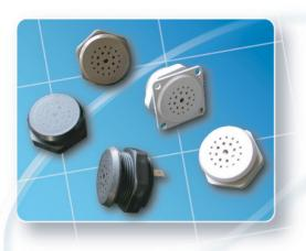
The standard series are based on the highest piezo technology and are considered as most robust series for industrial applications. The standard buzzers use a special shaped membrane (curved edge), which is fixed and glued into the housing. They are shock proof, as well as dust and waterproof (IP67). The different standard models cover a wide range of applications, offering functions such as continuous, intermittent, sweep and warbler, with a sound output of more than 100 dB(A).
