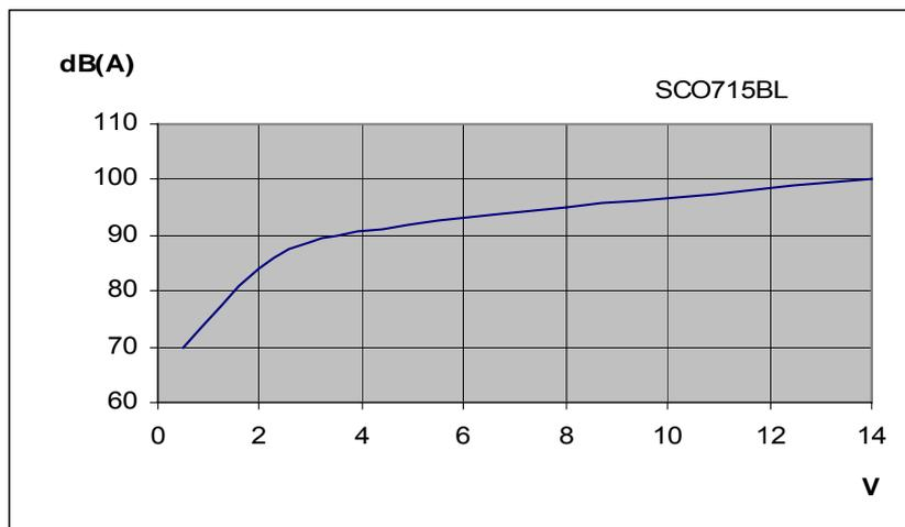
All measurements are made at 1 meter in free air at 21°C.
