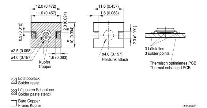
Anode and heatsink are electrically connected.
