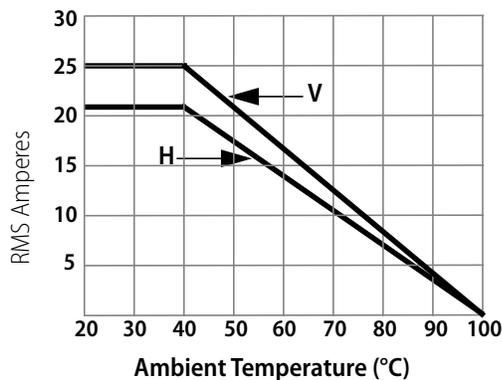
**V:** Heatsink mounted to a **vertical** surface
