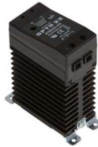
The HS Series features an integrated heatsink, which makes them so *cool*. These relays have less thermal resistance inside, so heat dissipates more easily than in a standard SSR mounted to the same heatsink. With the heatsink built-in, you don't have to select one from a catalog, and installation is much easier. Includes a DIN-rail adapter. See [page 13](#).
