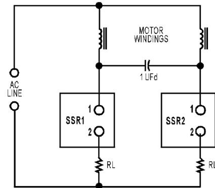
The resistors are unnecessary if the control circuit is designed to ensure that one SSR is off before the other SSR is on.
