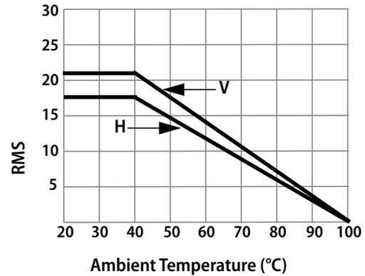
**V:** Heatsink mounted to a **vertical** surface
