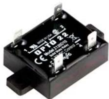
The Z Series employs a unique heat transfer system that makes it possible for Opto 22 to deliver a low-cost, 10-amp, solid-state relay in an all-plastic case. The push-on, tool-free quick-connect terminals make the Z Series ideal for high-volume OEM applications. Operating temperature: –40 °C to 100 °C. See [page 7](#).
