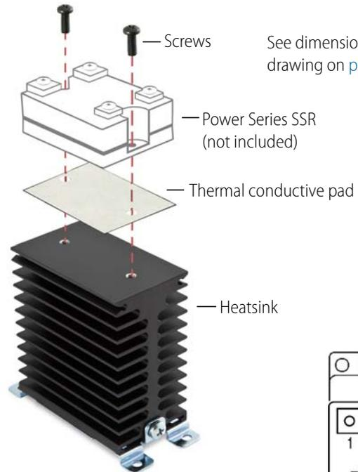
*NOTE: To take advantage of the cooling effect of natural air flow, mount the SSR/heatsink assembly to a vertical surface with the Opto 22 logo right side up as shown here.*
