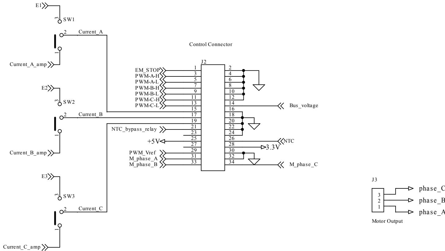
Figure 3. STEVAL-IPMNM5Q board schematic (3 of 5)
