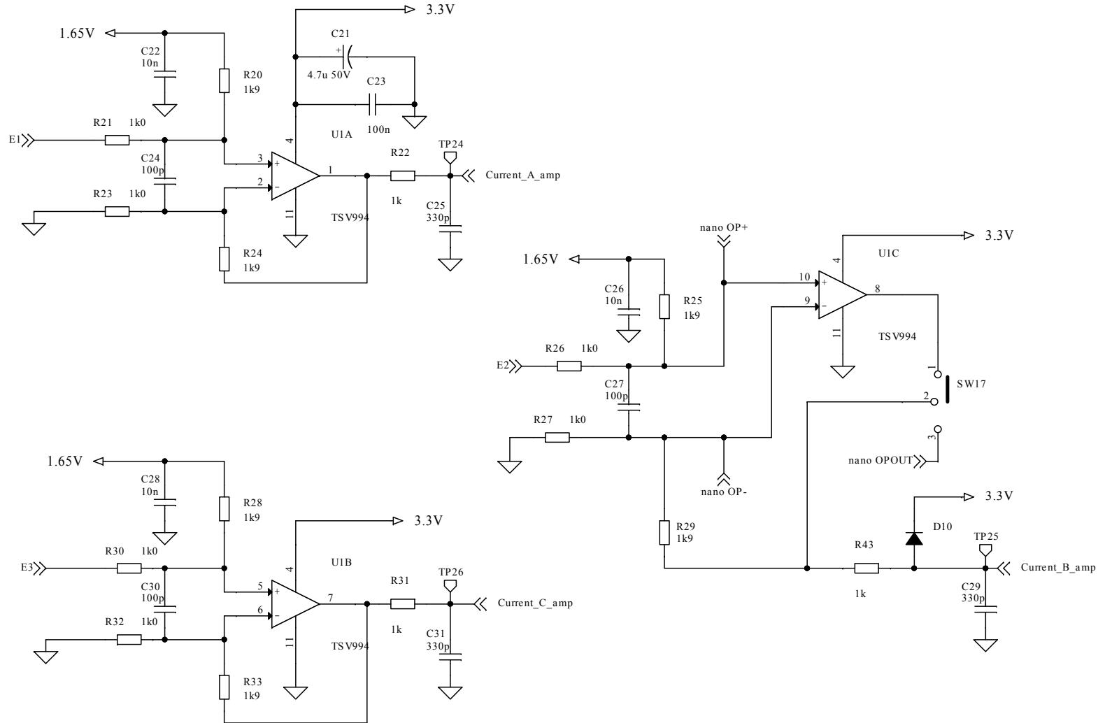
Figure 4. STEVAL-IPMNM5Q board schematic (4 of 5)
