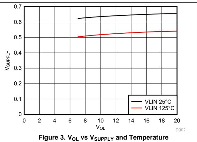
Figure 3.  $V_{OL}$  vs  $V_{SUPPLY}$  and Temperature
