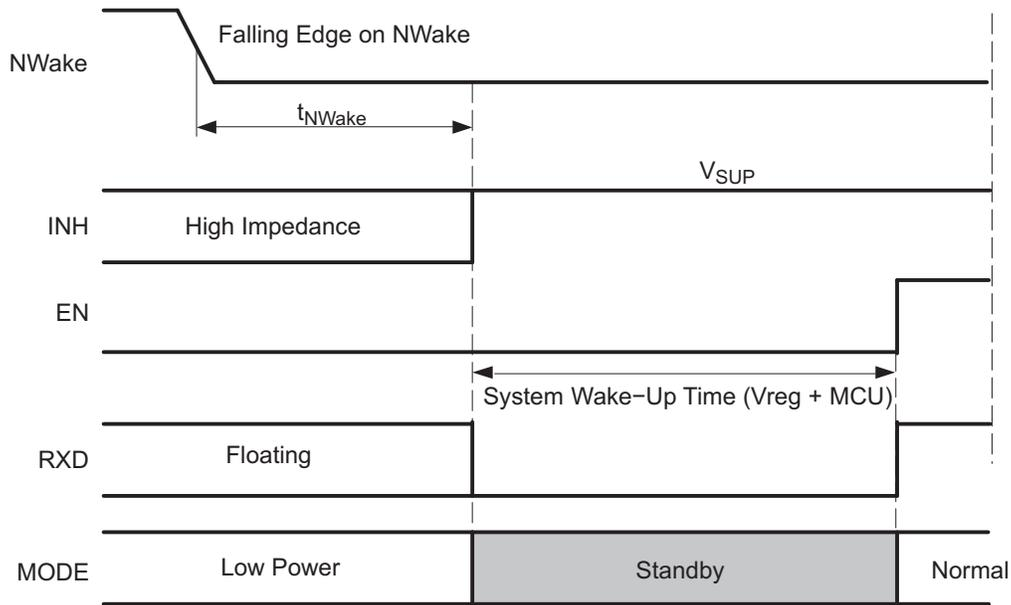
**Figure 6. Wake-Up Via NWake Timing Diagram**
