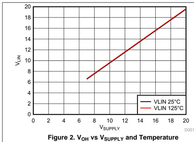
Figure 2.  $V_{OH}$  vs  $V_{SUPPLY}$  and Temperature
