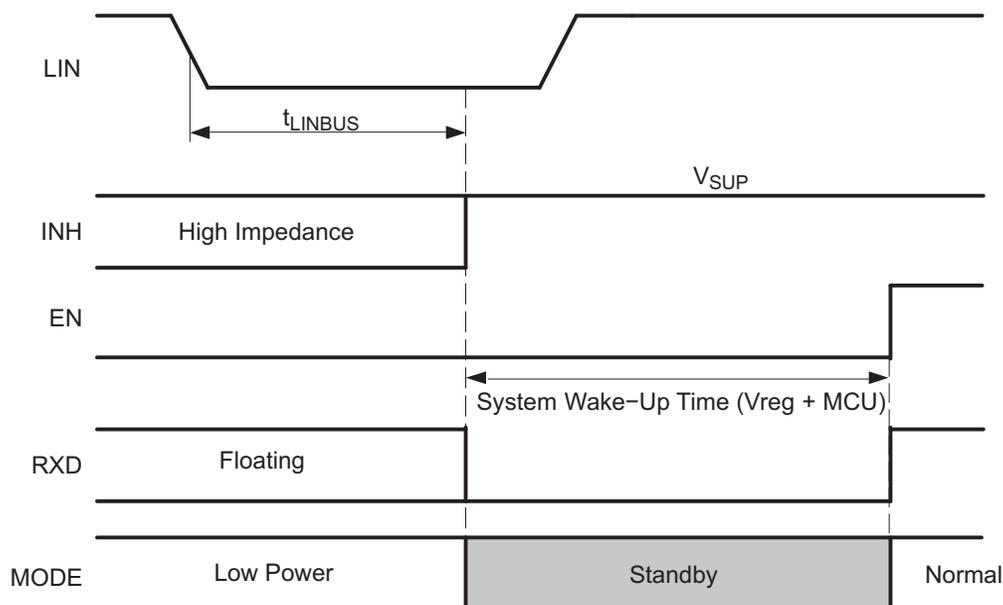
Figure 5. Wake-Up Via LIN Bus Timing Diagram
