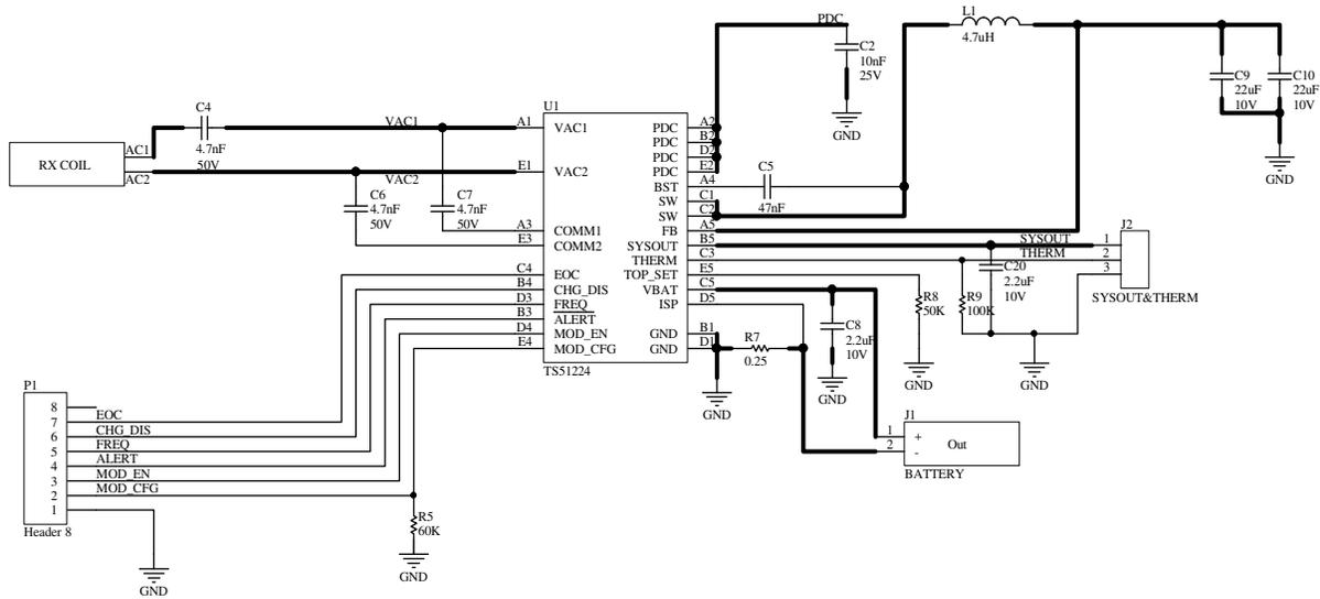
**Figure 7: Minimal PCB Area Configuration**
