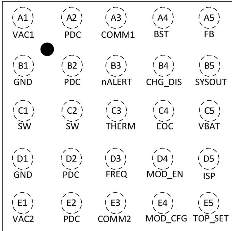
**Figure 1: TS51224 Ball Configuration**
