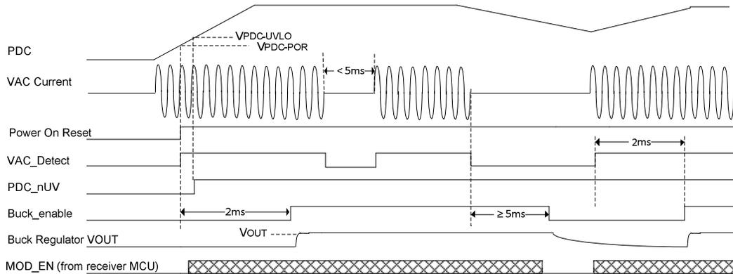
**Figure 5: VAC Signal Loss & Buck Control**
