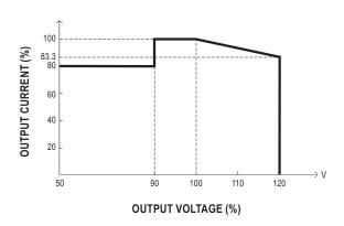
① The rated current should change with the Output Voltage Programming accordingly.
