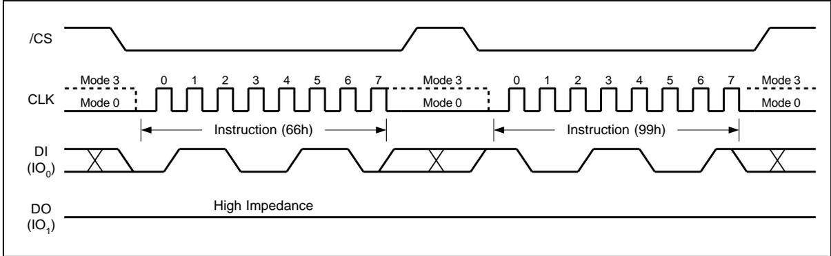
Figure 39a. Enable Reset and Reset Instruction Sequence
