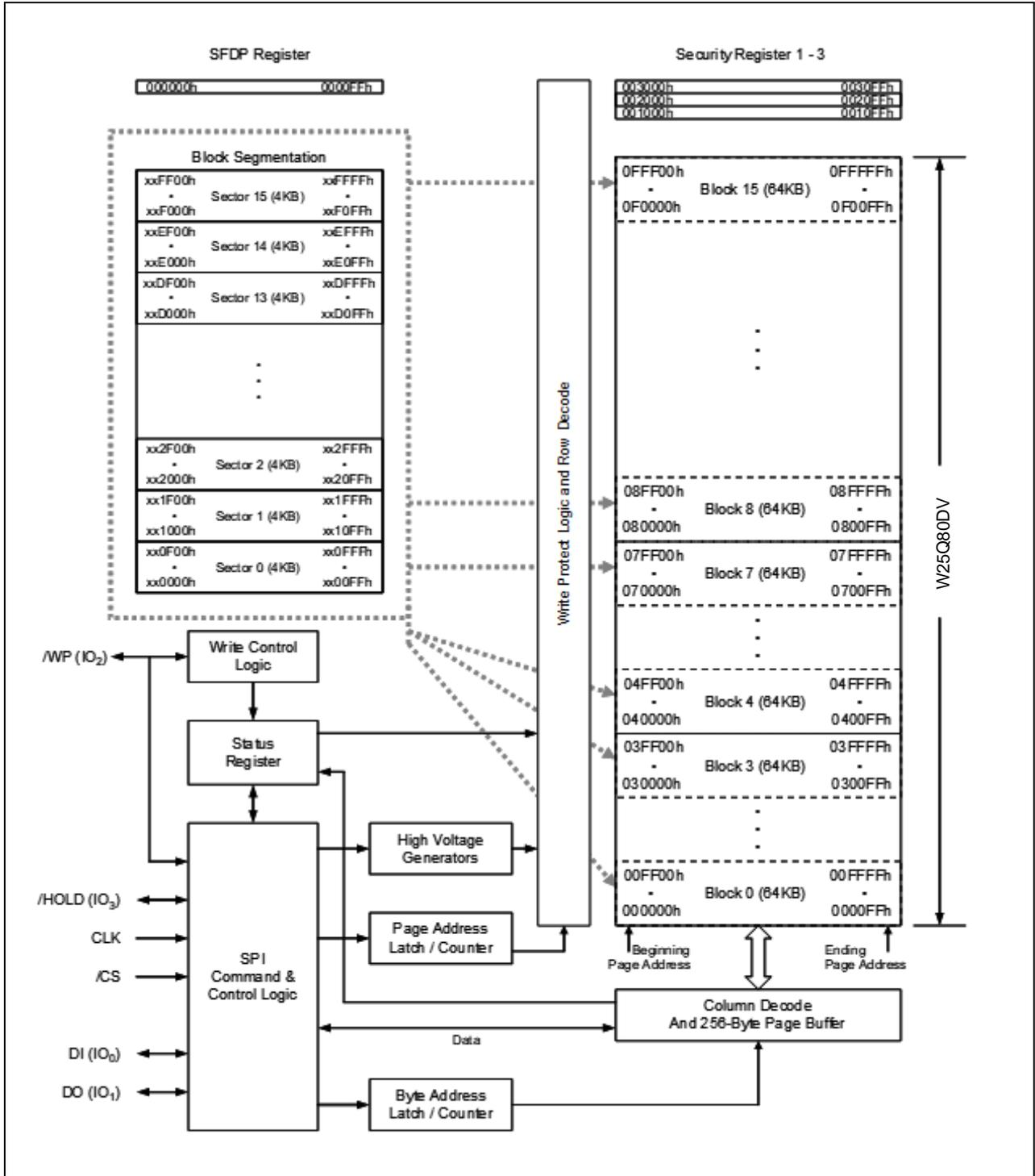
Figure 2. W25Q80DV Serial Flash Memory Block Diagram
