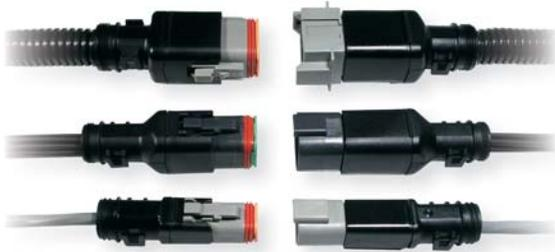
The Deutsch DT Series backshells are designed to snap onto and mate with all standard (basic plug and receptacles without modifications) DT Series connectors. The rigid, durable backshells offer a high level of protection and allow convoluted tubing to nest within the rear of the backshell. Straight (180°) and right angle (90°) versions and backshells with strain relief for jacketed cable are also available.
