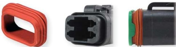
The DT P012 plugs provide enhanced front seal retention providing an ultra tight environmental seal. The enhanced seal retention keeps the seal in place during mating and unmating. The P012 modification requires an enhanced P012 wedgelock. Deutsch's P012 modification is available in 2, 3, 4, 6, 8, and 12 cavity arrangements.
