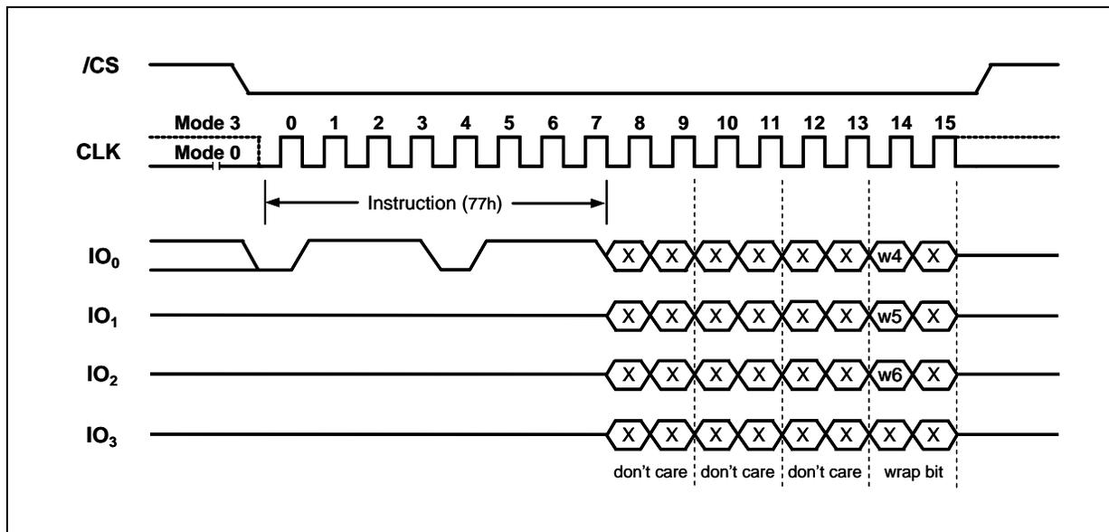
Figure 17. Set Burst with Wrap Instruction Sequence
