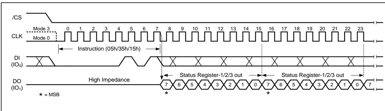
Figure 8a. Read Status Register Instruction (SPI Mode)
