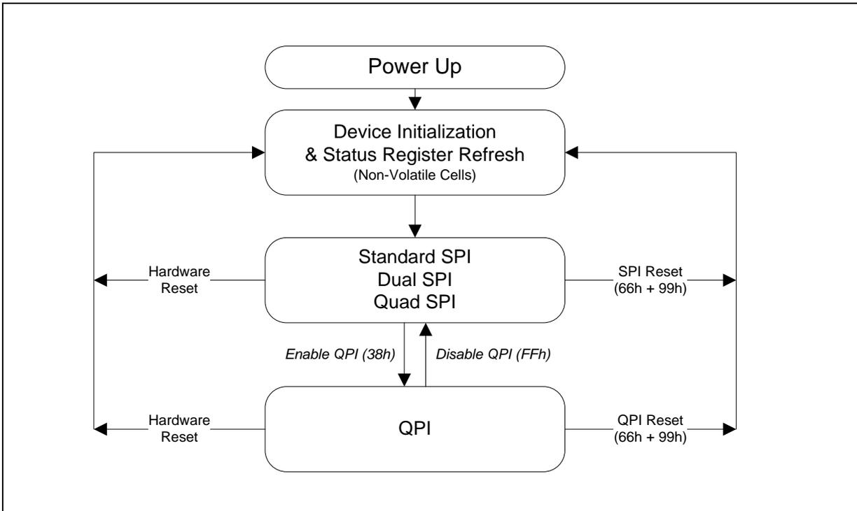
Figure 3. W25Q16JV Serial Flash Memory Operation Diagram
