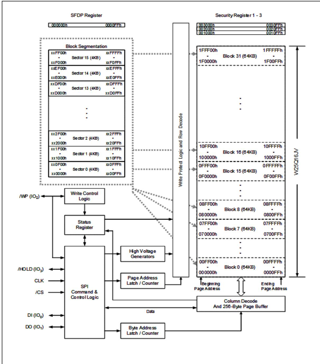
Figure 2. W25Q16JV Serial Flash Memory Block Diagram
