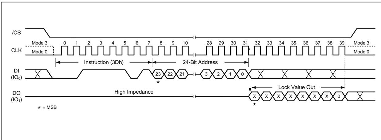
Figure 55a. Read Block Lock Instruction (SPI Mode)
