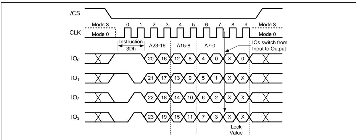
Figure 55b. Read Block Lock Instruction (QPI Mode)
